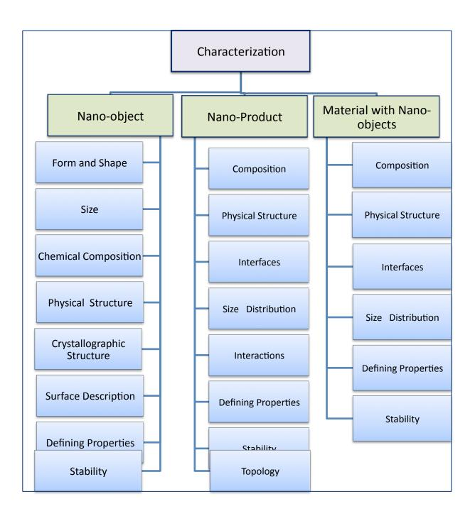
Figure 2. Schematic of the main information subcategories in the characterization of an individual nanomaterial.
