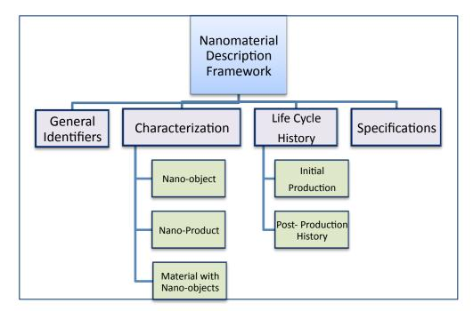
Figure 1. Schematic of the four main information categories and major subcategories of the Framework for a nanomaterial uniform description system.
