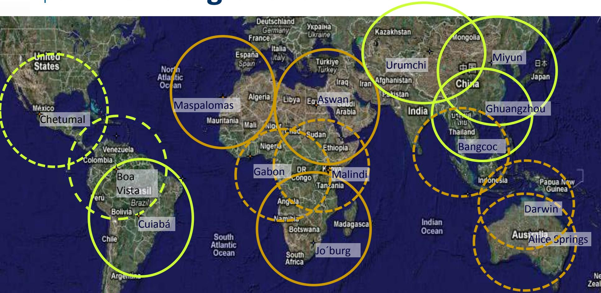
CBERS ground stations will cover most of the Earth's land mass between  $30^{\circ}\text{N}$  and  $30^{\circ}\text{S}$
