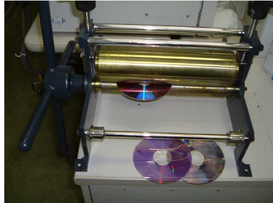
Roll mill to split DVD by applying pressure
