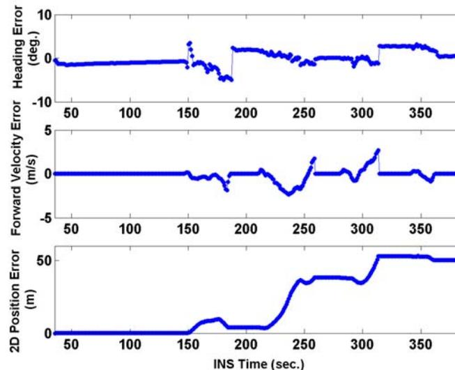
**Figure 12: Heading, Velocity and Position Estimation Error**
