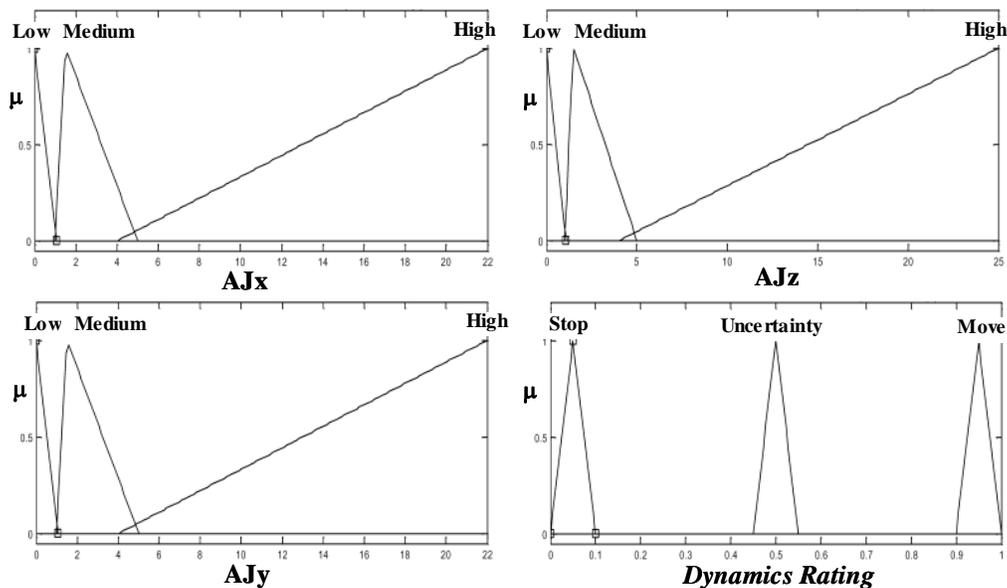
**Figure 3: Membership Functions used in Fuzzy Expert System**
