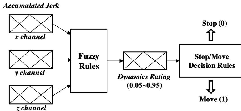
**Figure 2: Fuzzy Logic-based Vehicle Dynamics Identification System**
