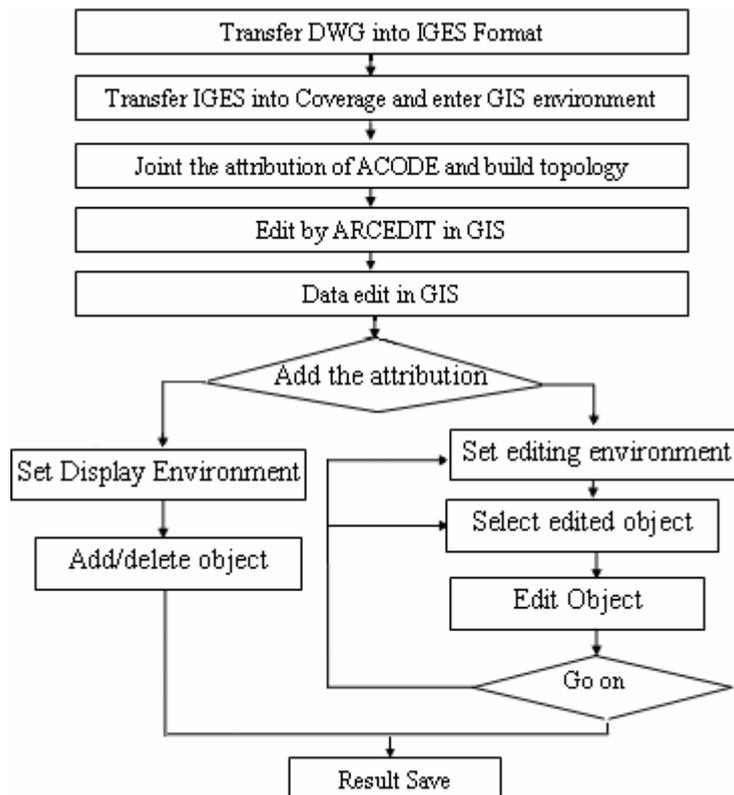
Figure 3. A illustration of data transform (transfer DWG file into GIS coverage)
