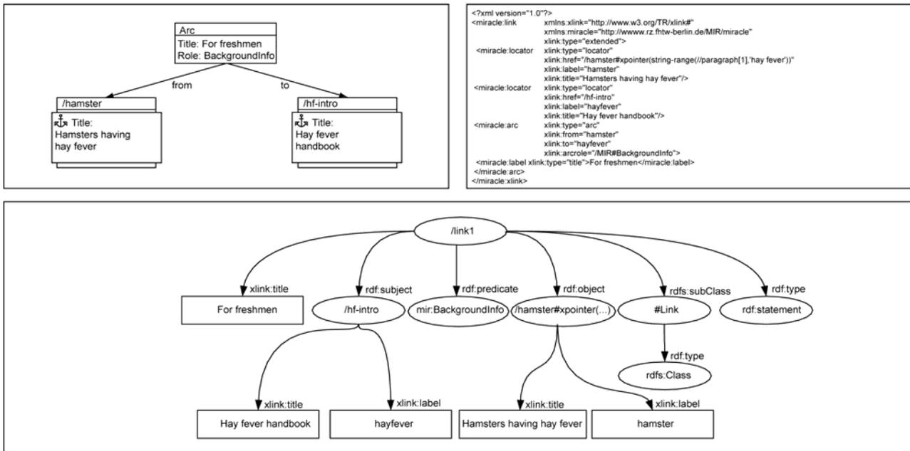
**Figure 2: Gaining a RDF hyperlink description from XLink**
